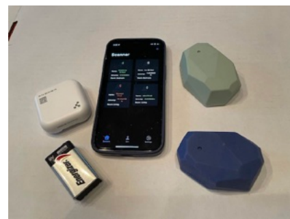
Fig 2. iPhone & two brands of commercially available beacons. 9V battery for scale.
